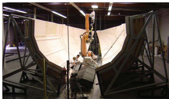
Technicians tending to Marie as she is machining massive part from Precision Board Plus
