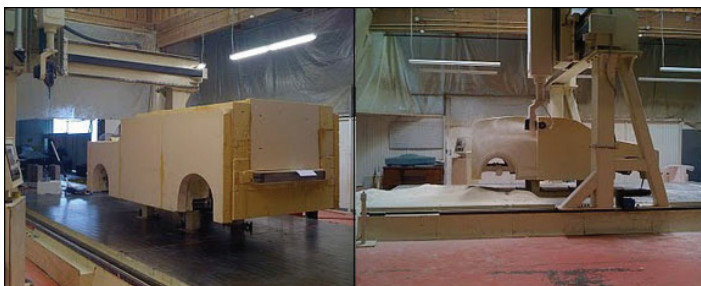
Precision Board Plus blocks mounted to steel substructure prior to the start of machining
