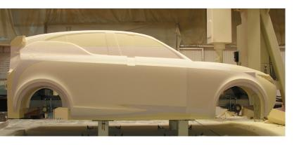
Precision Board Plus was created in 2008. The original chemical formula and manufacturing methods were redesigned to meet both the rigorous demands of an artist's creation and the machining standards of today's 5 axis milling machines.
