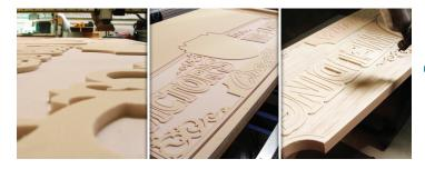
When they get a sandblasted job, such as the sign featuring the Aztec Calendar, they first CNC route **PBLT-15** to the desired depth of the background, before sandblasting. This allows the sandblaster to be used for a shorter period of time, freeing up an employee to work on another paying sign. After routing, the sign will get a quick sandblast to get the required texture.
