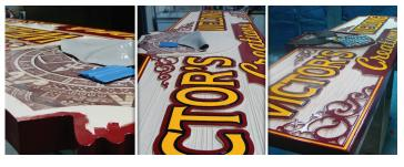
After priming and painting, Kevin the lead designer says they use 1-Shot lettering enamels "because of its vibrancy". In the case of the Aztec Calendar, a vinyl appliqué was applied under a separate piece of PBLT-15, to not only save time on hand painting, but to create a 3-D effect as well. As with all their signs, it was then coated with 2 coats of clear coat to preserve the quality and luster of the paint.
